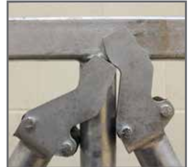
ABOVE: ERGONOMICALLY DESIGNED YOLK PREVENTS SWINGARM BINDING
