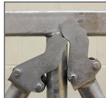
ABOVE: ERGONOMICALLY DESIGNED YOLK PREVENTS SWINGARM BINDING
