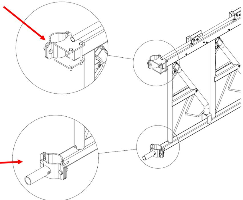
**Step 5:** Bolt handle mount to the lockup control pipe holder at desired location using 2 provided bolts. Install 2 self-tapping screws on each side. Handle can be mounted at any head opening.
