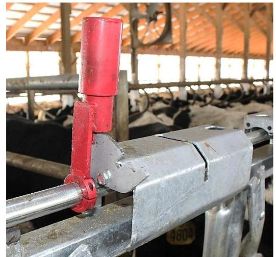
Slide Control Rod Connector on before installing next lockup section
