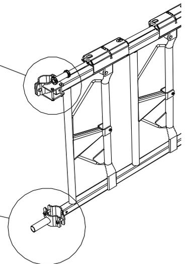
**Step 6:** Slide the control connector onto the control rod *prior* to installing the next lockup section. Once all sections are installed, rotate the control rods until *all* the flippers are perfectly horizontal. Tighten connectors using supplied wrenches. **Note: It is critical for proper function and performance to have all control rod flippers aligned to the same horizontal plane.**
